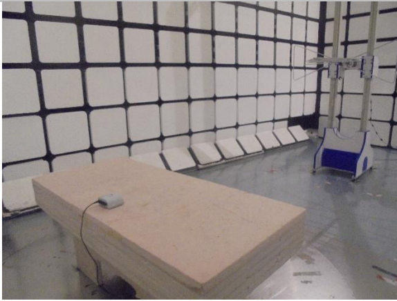
Radio-frequency radiated emissions 30 MHz to 1 GHz
