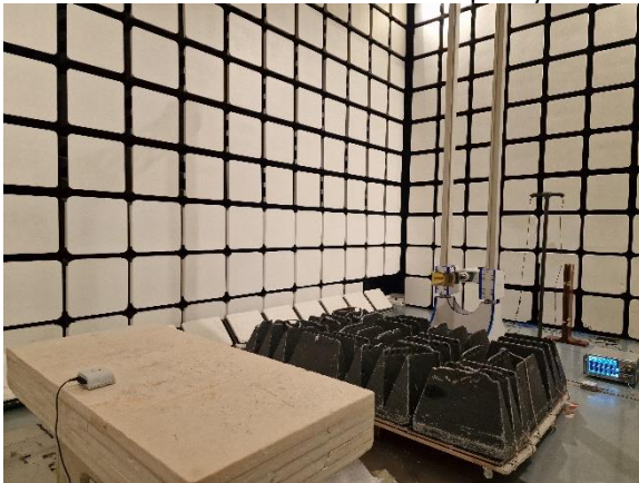
Radio-frequency radiated emissions 1 GHz to 13.5 GHz
