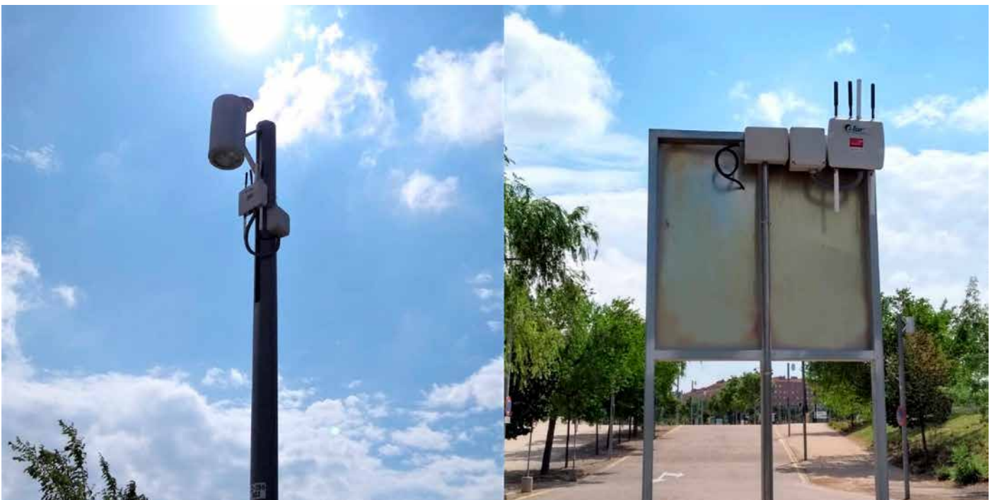
Two Meshlium scanners are installed at the access of the park
