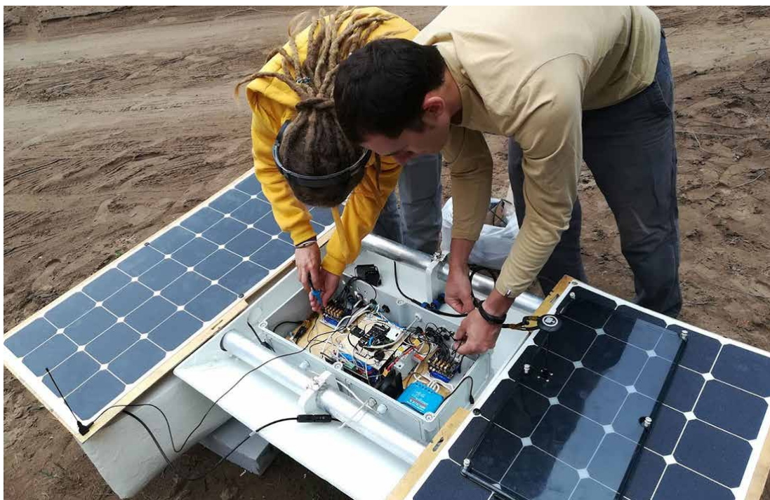
Installing Wasp mote Smart Water sensor platform in the drone
